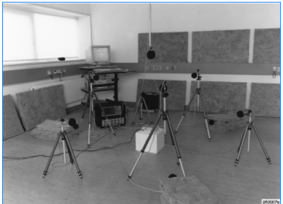
Fig. 4 Sound power determination in an office according to ISO 3744. With the reference sound source Type 4204, which can be seen behind the tape streamer; the acoustic properties of the room can be determined. To obtain sufficient absorption, absorption material had to be installed
